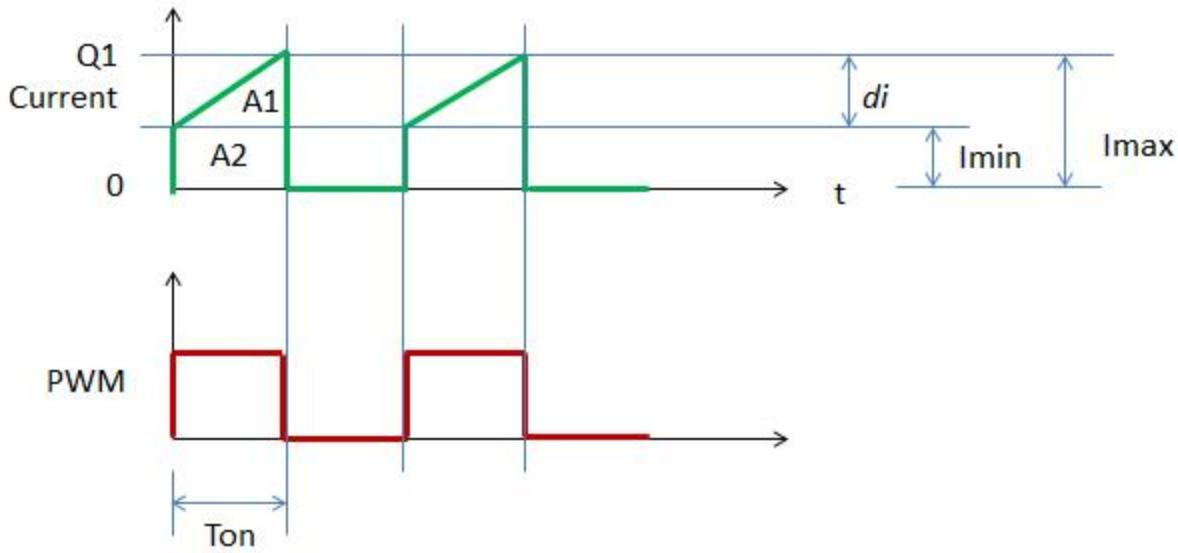
The RMS current of the switch is the sum of the RMS of the area \$A\_1\$ and \$A\_2\$. \$A\_1\$ is a triangle while \$A\_2\$ is rectangle.
