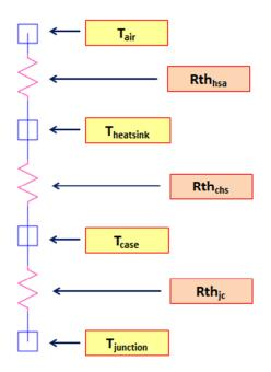
Below is an equation relating the temperatures and thermal resistances.
