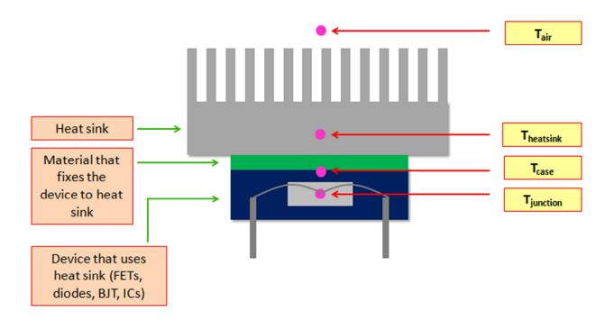
In between temperatures, there is a thermal resistance as illustrated below.
