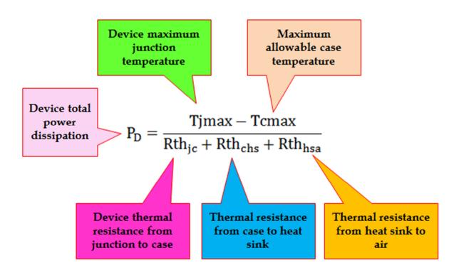
The heat sink thermal resistance and what we are after of is the variable  $Rth_{hsa}$ . By simple rearranging of the above equation will give the  $Rth_{hsa}$ .
